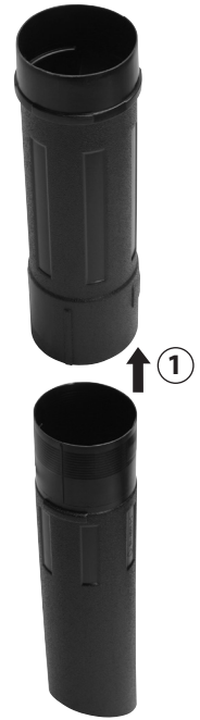
Figure 3-8: Connecting lower and upper vacuum tube together
